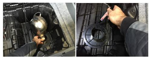
Drill the hole (about 7 centimeters – most drillers have 68mm size) and also drill small holes where you can screw the flange from the outside (screws are supplied by us):
