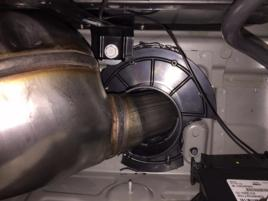
On BMW G30 / G31 5series (depending on the accessories of the BMW) the space next to the batterie in the middle of the trunk might fit perfectly. Because the space is very limited there, you might not be able to mount / use the flange / ring as well – you might have to mount it without.. The following pictures do show a G30 installation – second picture shows the outlet-tube of the soundbooster from underneath the car:
