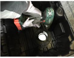
Glue the Soundbooster-pipe into the flange with regular silicone or dual-component adhesive. Then put enough silicone around the hole so it is waterproof if you put the flange with the soundbooster on it:
