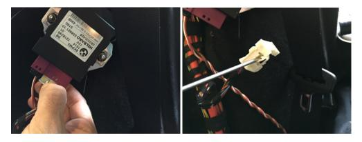
Remove the red pin of the drilled BUS-Cable pair first (on G-modells the yellow cable with the black line) – you can remove the pins by holding down the spring-lip on the side through the hole with a small screwdriver or a paperclip:
