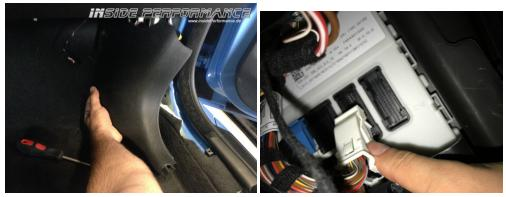
Our harness is long enough to go to the footwell compartment. To reach this place with the harness, just remove (pull up) the door entry covers as shown in the following picture and put the harness below the floor:
