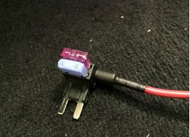
Connect our fuse holder to the power wire of the harness (red) and plug the fuse-holder into the socket where you removed the cigarette-lighter fuse:
